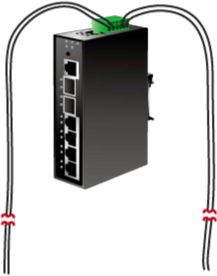
DC/DC Power Failure
